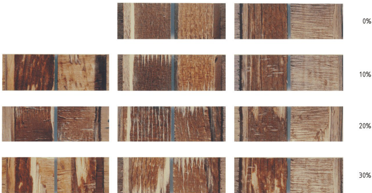
Figure A.1 — Wood fibre failure 0 % to 30 % reference illustrations
