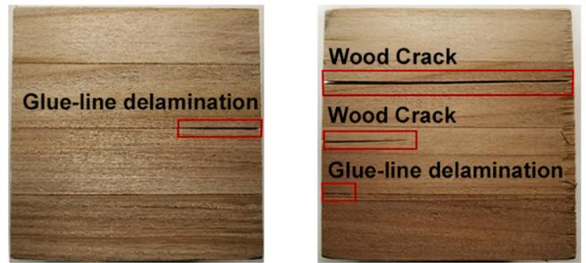
Fig. 9. Typical failure mode of delamination test.
