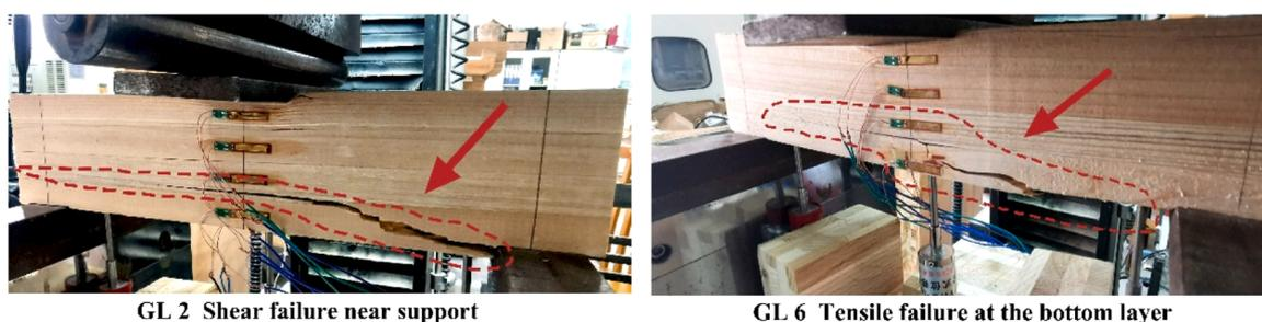
Fig. 14. The typical failure modes of normal Chinese fir glulam.
