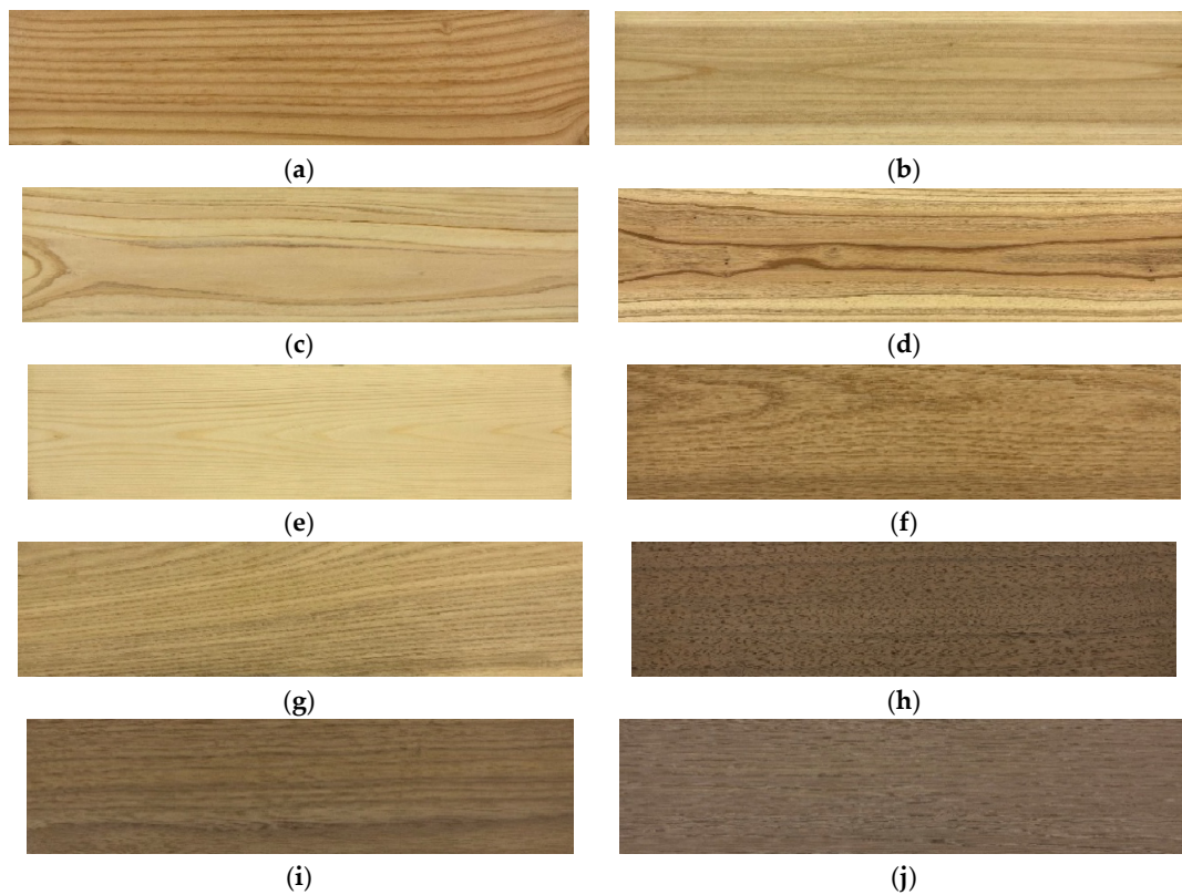
Figure 1. Wooden materials used in this study: (a) Douglas-fir ( Pseudotsuga menziesii (Mirb.) Franco); (b) Chinese fir ( Cunninghamia lanceolata (Lamb.) Hook.); (c) Japanese cypress ( Chamaecyparis obtusa (Siebold & Zucc.) Endl.); (d) Japanese cedar ( Cryptomeria japonica (Thunb. ex L.f.) D.Don); (e) Norway spruce ( Picea abies (L.) H. Karst.); (f) Northern red oak ( Quercus rubra L.); (g) American ash ( Fraxinus americana L.); (h) Black walnut ( Juglans nigra L.); (i) Veneered plywood; (j) Decorative particleboard.
