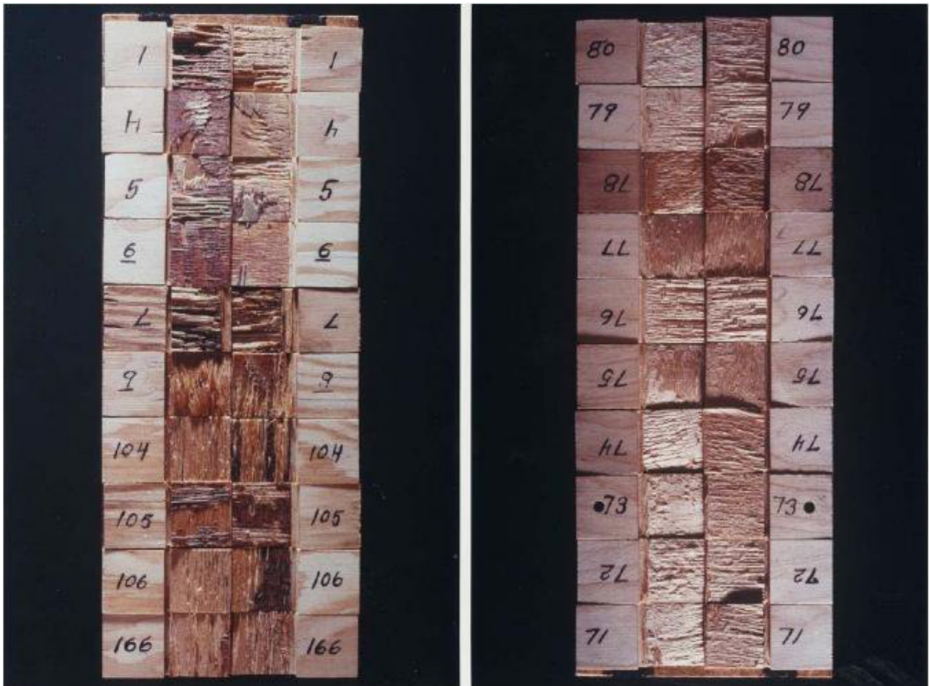
FIG. X1.1 Visually Estimating the Percentage of Wood Failure in Standard Adhesively Bonded Specimens (Left) Three-ply, Douglas-fir, Phenol-formaldehyde adhesive. (Right) Three-ply, Yellow-birch, Urea-formaldehyde adhesive.
