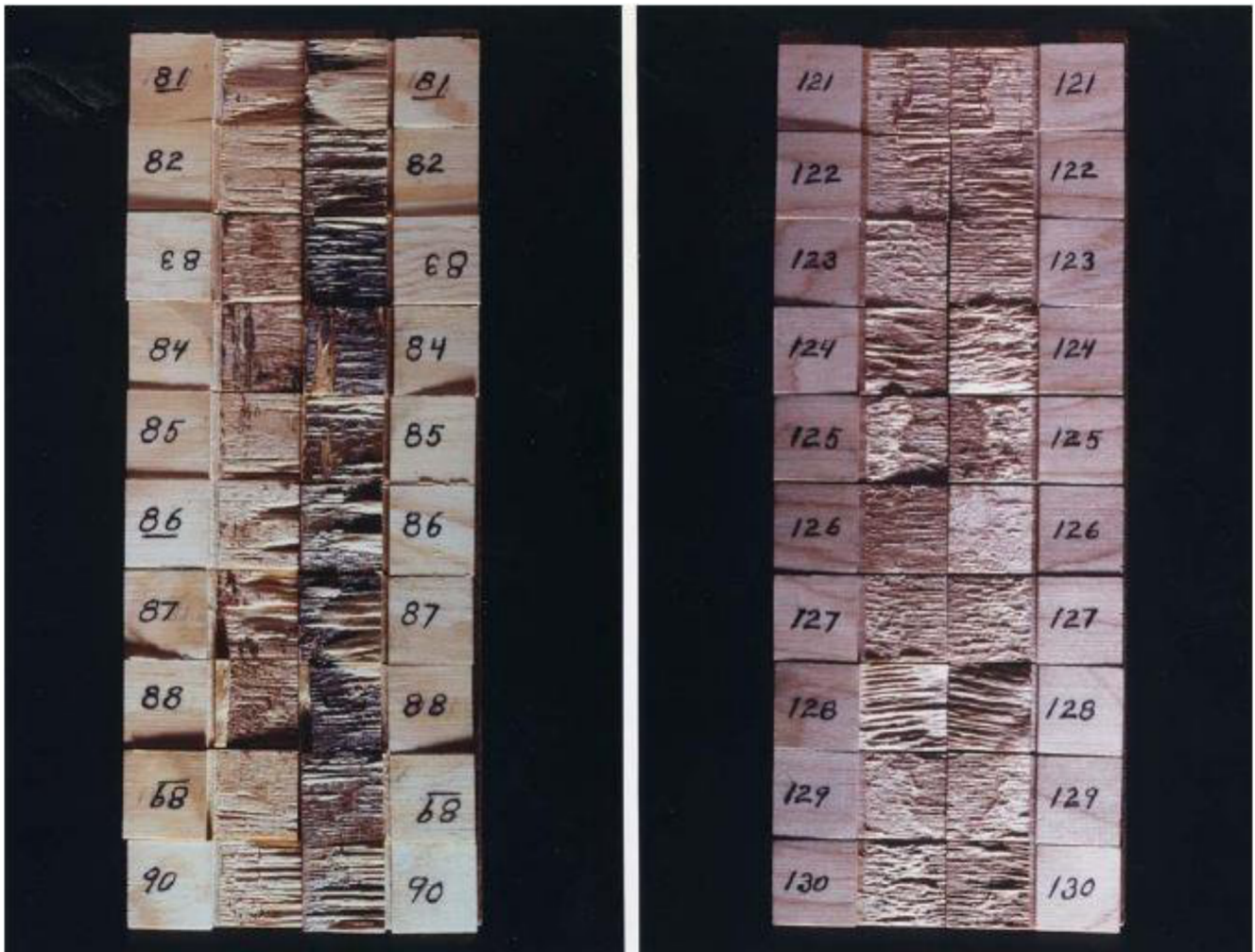
FIG. X1.2 Visually Estimating the Percentage of Wood Failure in Standard Adhesively Bonded Specimens (Left) Three-ply, Southern pine, Phenol-formaldehyde adhesive. (Right) Two-ply, Yellow-birch, Urea-formaldehyde adhesive.
