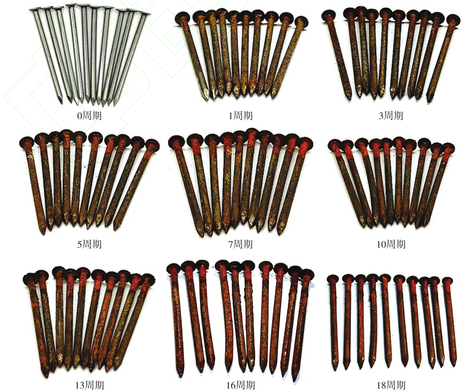
图 6 各周期钉锈蚀图 Fig. 6 Corrosion diagrams of nails in different cycles
