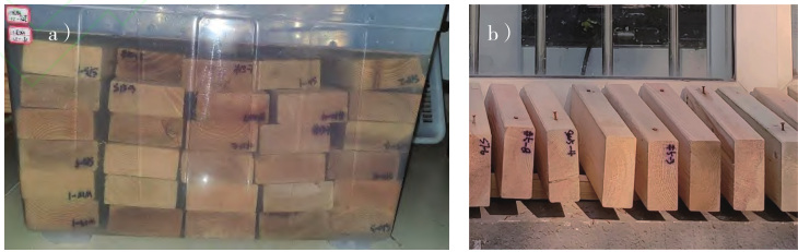
图 2 试件浸泡(a)和晾晒(b)示意图 Fig. 2 Schematic diagram of specimen soaking (a) and drying (b)
