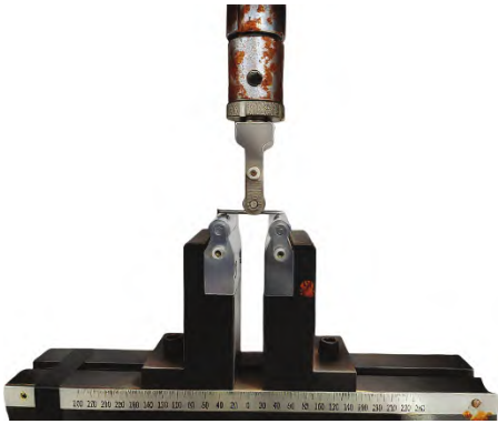
图 4 钉抗弯试验加载示意图 Fig. 4 Schematic diagram of the nail bending test loading
